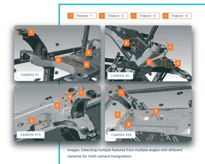
Mapvision's patented multi-camera technology enables Mapvision Q to internally evaluate its own measurement process by comparing results from multiple triangulations. Even in case of a camera obstruction, the system can detect and isolate the problem while continuing to provide uncompromised results from other triangulations – providing reliable, uninterrupted performance at all times.
